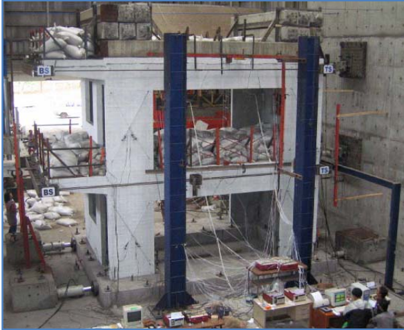
Fig. 6: PC-wall panel with precast/prestressed half slab full-scale model
